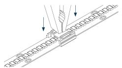
2 | Insert Uniform LED tape into connector. (Confirm polarity of LED strips match each other)
