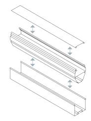
Install LED strip centered in groove of top channel and attach lens. If using optical lens, slide in one at a time.
