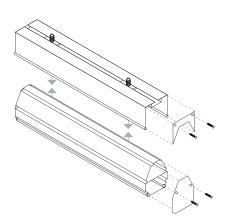
Thread channel couplers back onto T-screws and then position T-screws to align with the marked suspension points from the previous step.
