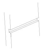
Insert disposable cover into channel, measure, and cut to length.
