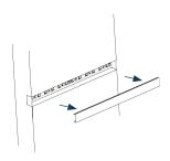
Tape and mud over mounting surface, bring mud flush to edge of disposable cover.
