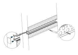
Install LED strip into channel and route wire back to remote power supply location.
