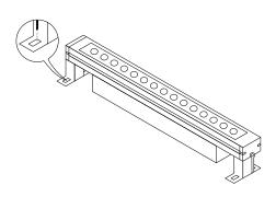
Re-position the fixture and rotate it to one side. Locate the marked or pre-drilled holes. Attach with appropriate hardware.
