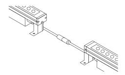
Connect the first unit to the appropriate line voltage source. Make sure an end cap is on the last, unused integrated cable connector.
