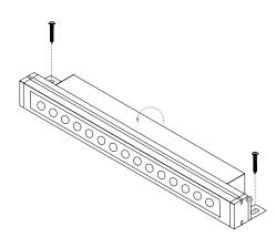
Rotate fixture back to proper position. Tighten stand off pivot bolt to secure desired angle.
