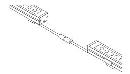
Connect the first unit to the appropriate low voltage source. Make sure an end cap is on the last, unused integrated cable connector.
