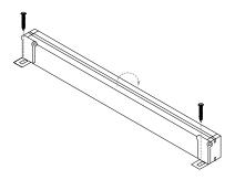
Fully rotate the fixture to the other side to expose the remaining holes. Attach with appropriate hardware.
