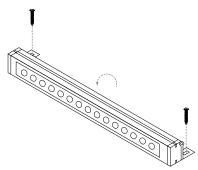
Rotate fixture back to proper position. Tighten stand off pivot bolt to secure desired angle.
