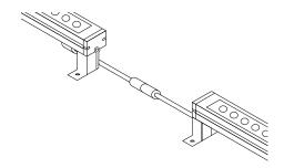
6 Connect the first unit to the appropriate low voltage source. Make sure an end cap is on the last, unused integrated cable connector.
