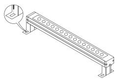
Re-position the fixture and rotate it to one side. Locate the marked or pre-drilled holes. Attach with appropriate hardware.
