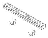
Connect each of the desired units in series using integrated cables or provided connectors.
