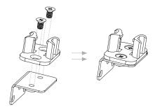
Place the tape with angle mounting clips to desired location and drill holes.
