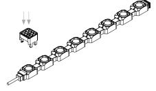
Place the tape with angle mounting clips to desired location and drill holes.
