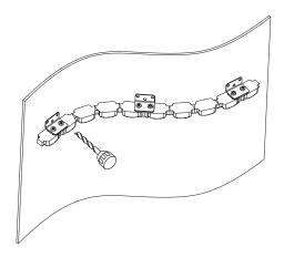
Push narrow section of tape between the LEDs into the plastic clip
