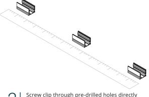
Screw clip through pre-drilled holes directly into mounting surface.
