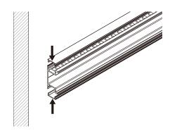
Attach end caps and secure using included screws.
