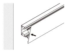
$2 \mid \text{Secure channel to wall using pre-drilled holes.}$
