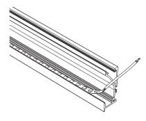
(Optional) If installing the channel with spring clips, slide the spring clips used for this section prior to installing end caps.
