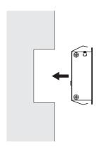
Thread included screw through clip and back of channel.
