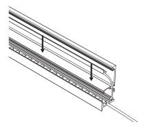
Slide leader cable through end cap with hole and install end caps on both ends of channel.
