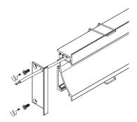
Remove lens and install LED strip into channel with leader cable pointed towards power source.
