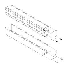
Snap top and base channels together at desired angle.
