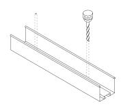
Screw through pre-drilled holes directly into mounting surface.
