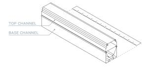
After cutting detach channels using a tool and remove lens from channel.
