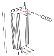
4 Confirm mounting postion and wiring figuration are as desired.
