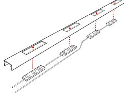
5 Run power feeds through bottom half of channel then connect two halves together
