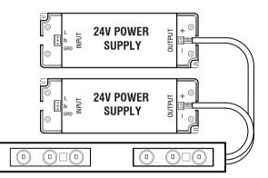
6 Connect primary side of power supplies to AC line voltage power source
