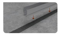
Press fit BrightLinx into the channel.
