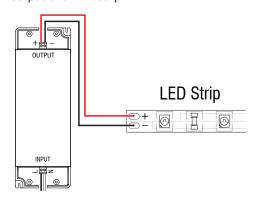
Optional: connect plug-in power feed to power supply in lieu of hardwire connection
